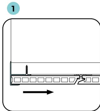
Begin by fixing the corner profile into place before installing the first board.
