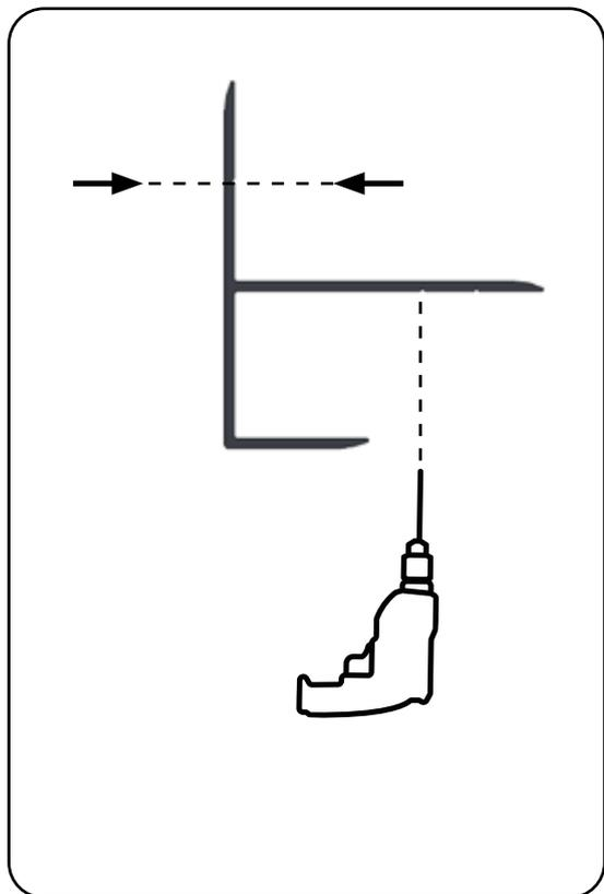
The multi-functional corner profile can have holes drilled into it in different places, depending on how it is used on the cladding.
