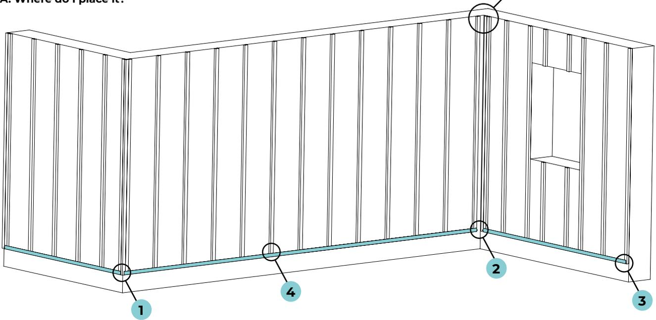
When positioning the start profiles, maintain the distances specified below in order to leave room for the multi-functional corner profile.
