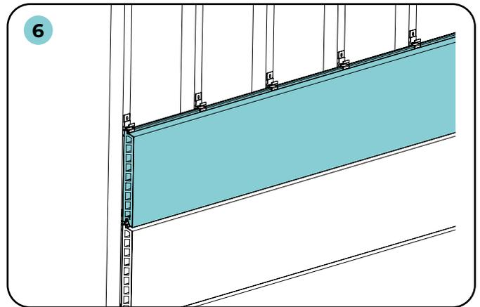
5. Fit the next board in the same way, continuing up to the top of the structure.
