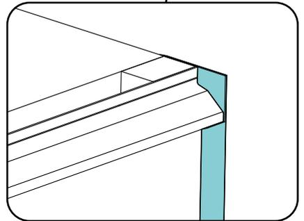
To make the join between profiles at corners, cut both end profiles at an angle of 45°
