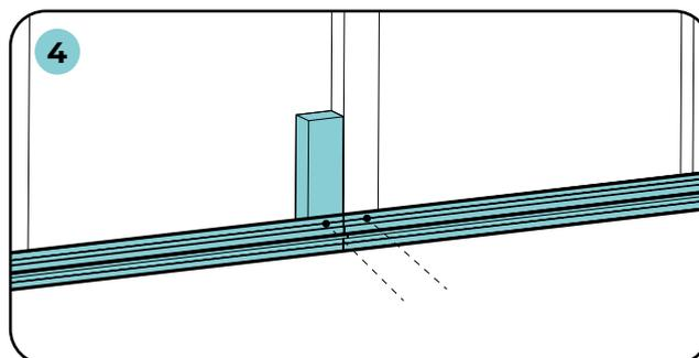
To butt a profile, add a second cleat to the structure at that location to help fix each end of the profile firmly in place.
