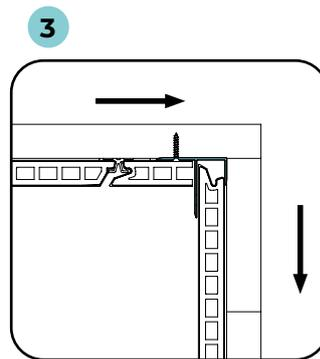
Affix the corner profile before installing the last board on this wall. Then fix the board in place using a Silvadec® special composite screw.
