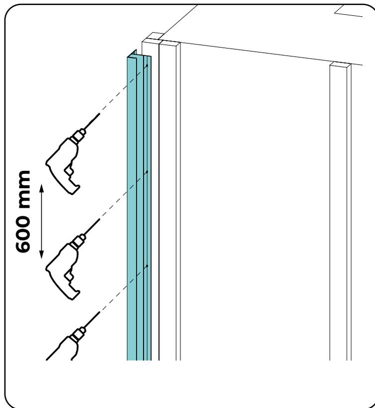
Drill into the groove of the profile, then screw the profile onto the cleat, leaving a gap of 600 mm between adjacent screws.
