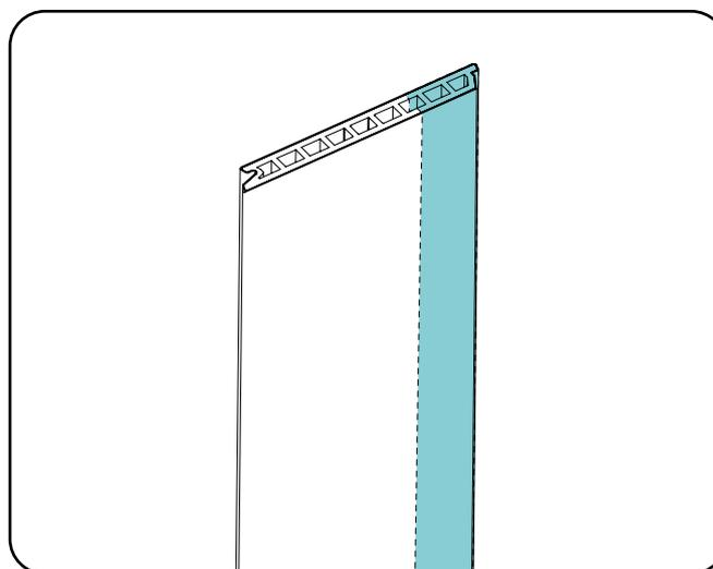
Again, the edge of the final board can be removed, to fit the cladding to the length of the wall
