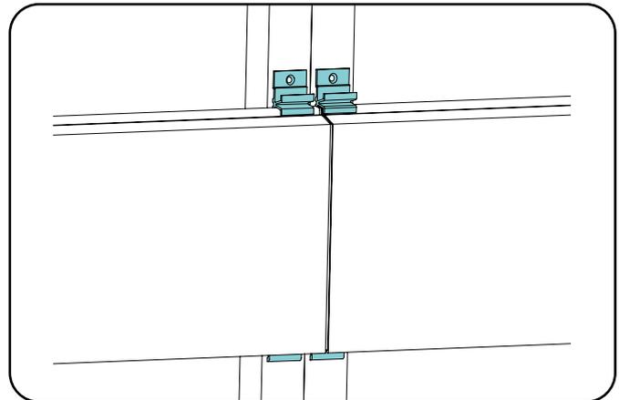
Reminder: The boards must be fitted to the cleats with an overhang not exceeding 50 mm.
