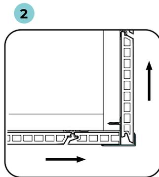
Affix the corner profile after the last board on this wall has been installed.
